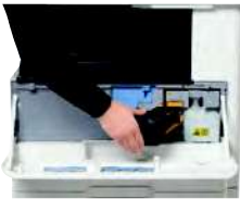
Easy replaceable toner container with a high yield of 15,000 pages.
