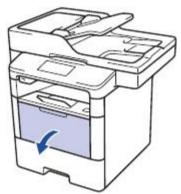
Pull out the MP tray support (1) and unfold the flap (2).
