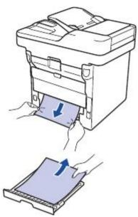
Remove paper that may have jammed under the machine due to static electricity.
