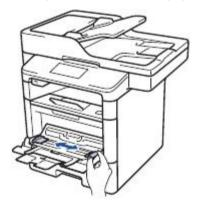
Load paper with the printing surface face up in the MP tray. When you use Letterhead or Preprinted paper, load the paper in the correct orientation as shown in the illustrations.
