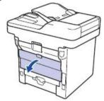
Pull the green levers at the left and right sides toward you to release the fuser cover.
