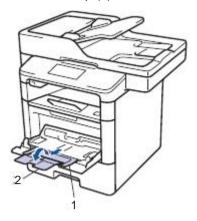
4 Slide the MP tray paper guides to fit the width of the paper you are using. If the paper guide on the right side has a lever, press it and slide the paper guide.
