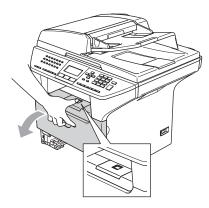
Slowly take out the drum unit and toner cartridge assembly. The jammed paper may be pulled out with the toner cartridge and drum unit assembly, or this may release the paper so you can pull it out of the paper tray opening.
