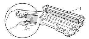
When you find the substance on the drum surface that matches the print sample, gently dab the surface of the OPC drum with a cotton swab that is lightly dampened with isopropyl alcohol.
