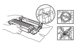
5 Put the drum unit and toner cartridge assembly back in the machine.
