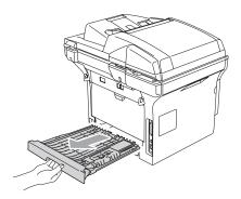
Pull the jammed paper out of the machine or the duplex tray.
