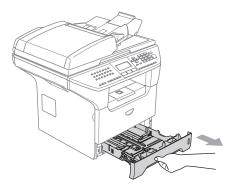
While pressing the blue paper-guide release lever (1), slide the paper guides to fit the paper size. Make sure that the guides are firmly in the slots.
