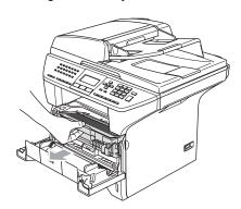
3 Hold down the lock lever on the right and take the toner cartridge out of the drum unit.
