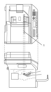
4 Put the drum unit and toner cartridge assembly back into the machine.
