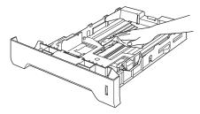
5 Re-load the paper and put the paper tray firmly back in the machine.
