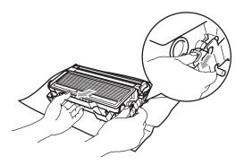
4 Put the toner cartridge back into the drum unit until you hear it lock into place. If you put it in properly, the lock lever will lift automatically.
