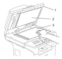
In the ADF unit, clean the white plastic bar (1) and the scanner glass strip (2) under it with isopropyl alcohol on a lint-free cloth.
