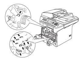
Gently clean the laser scanner window (1) by wiping it with a clean soft, dry lintfree cloth. Do not use isopropyl alcohol.
