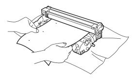
Turn the white gear on the drum as you check the surface of the OPC drum (1).
