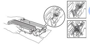
8 Put the drum unit and toner cartridge assembly back in the machine.
