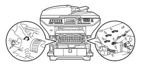
3 Clean the corona wire inside the drum unit by gently sliding the blue tab from right to left and left to right several times.
