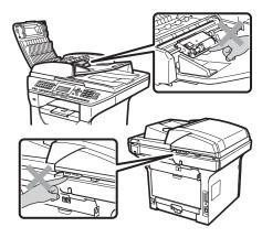
When you move the machine, grasp the side hand holds that are under the scanner.
