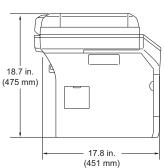
Weight With Drum/Toner Unit: 40.3lb (18.3kg) (MFC-8480DN)
