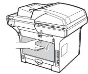
4 Pull the tabs at the left and right hand sides toward you to open the fuser cover (1).
