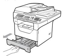
While pressing the blue paper-guide release lever (1), slide the paper guides to fit the paper size you are loading in the tray. Make sure that the guides are firmly in the slots.
