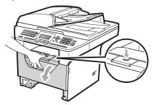
4 Slowly take out the drum unit and toner cartridge assembly. The jammed paper may be pulled out with the drum unit and toner cartridge assembly, or this may release the paper so you can pull it out of the paper tray opening.
