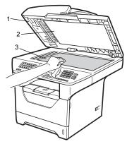
In the ADF unit, clean the white bar (1) and the scanner glass strip (2) underneath it with a soft lint-free cloth moistened with water.
