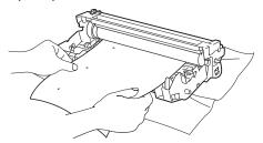
5 Turn the drum unit gear by hand while looking at the surface of the OPC drum (1).
