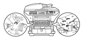
3 Push down the blue lock lever and take the toner cartridge out of the drum unit.
