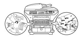
3 Push down the blue lock lever and take the used toner cartridge out of the drum unit.
