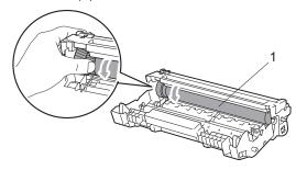
6 When you have found the mark on the drum that matches the print sample, wipe the surface of the OPC drum with a dry cotton swab until the dust or glue on the surface comes off.
