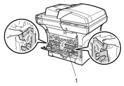
5 Pull the jammed paper out of the fuser unit.
