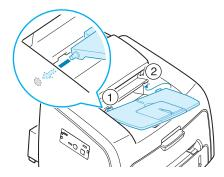
Fold out the extender, if necessary.
