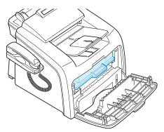
**2** Remove the starter toner cartridge from its bag. Gently roll the cartridge 5 or 6 times to distribute the toner evenly inside the cartridge.
