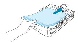
You can load letterhead paper with the design side face down. The top edge of the sheet with the logo should be placed at the front side of the tray.
