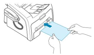
For envelopes, load a sheet with the flap side face down and with the stamp area on the top left side.
