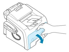
Pull the toner cartridge out and gently roll the cartridge 5 or6 times to distribute the toner evenly inside the cartridge.
