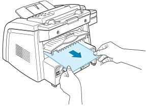
Printing from the manual feeder to the rear output slot provides the **straight paper path**. Using the rear output slot might improve the output quality with the following:
