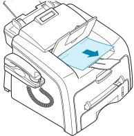
If there is any resistance and the paper does not move when you pull or if you cannot see the paper in the front output tray, continue to step 3.
