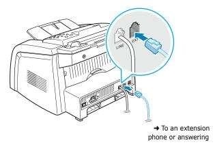
UK users should plug the cord of the extension phone into the supplied TAM lead and plug the cord of the TAM lead into the **EXT** jack on the back of your machine.
