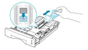
**2** After inserting paper into the tray, slide in the guide until it lightly touches the end of the paper stack.
