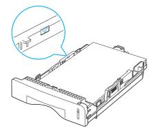
**6** Insert and slide the paper tray back into the machine.
