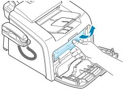
**3** Unpack the new toner cartridge and gently roll it horizontally four or five times to distribute the toner evenly inside the cartridge.
