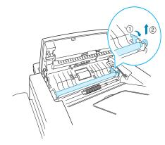
4 Wipe the roller surface with a soft cloth dampened with water.
