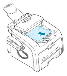
**4** Close the control panel. Then load the documents back into the ADF.
