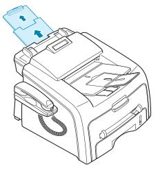
3 Load the document(s) to be scanned face down into the ADF (Automatic Document Feeder) and adjust the document guides.
