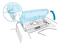
**3** Remove the control panel from the machine by disconnecting the hinge on the right.
