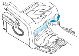
**3** With a dry lint-free cloth, wipe away any dust and spilled toner from the toner cartridge area and the toner cartridge cavity.
